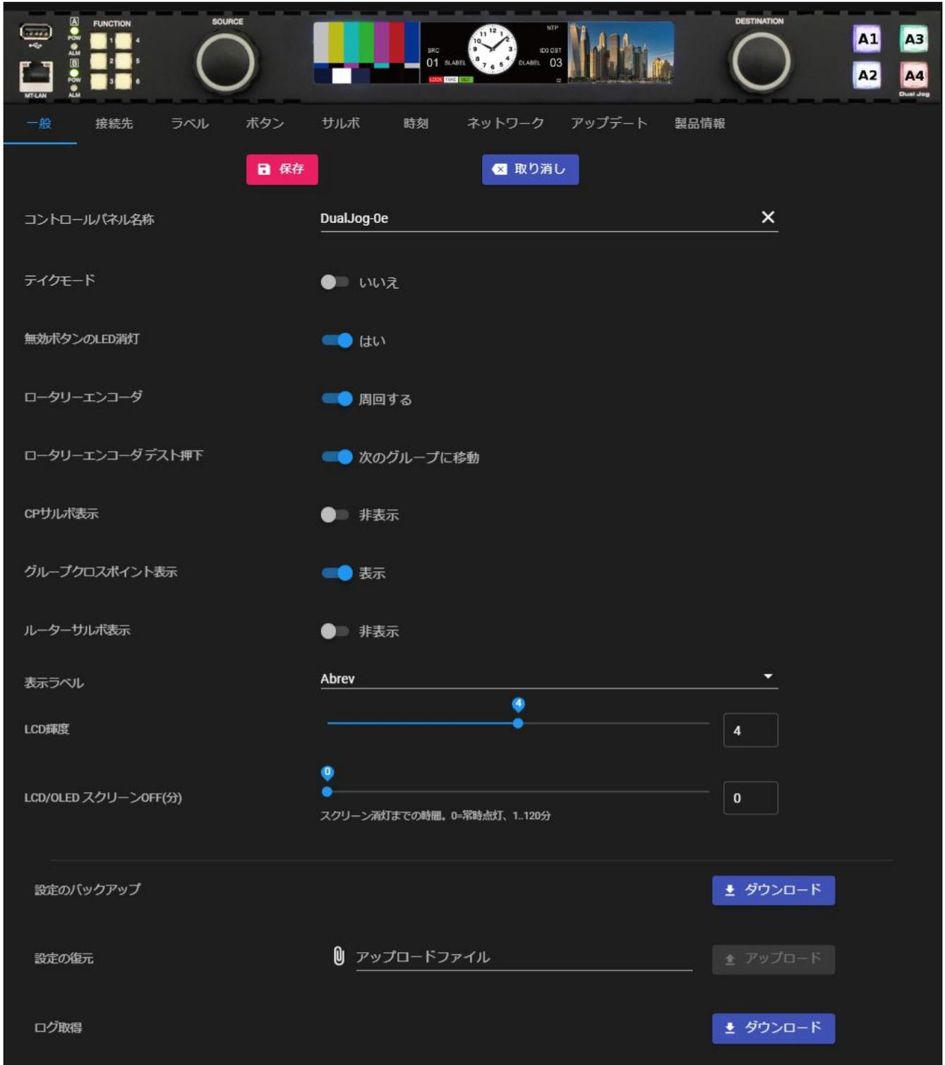
The screenshot displays the '一般' (General) settings tab for the DualJog control panel. The interface includes a top navigation bar with tabs for '一般', '接続先', 'ラベル', 'ボタン', 'サルボ', '時刻', 'ネットワーク', 'アップデート', and '製品情報'. Below the navigation bar are '保存' (Save) and '取り消し' (Cancel) buttons. The settings are organized into several sections:
